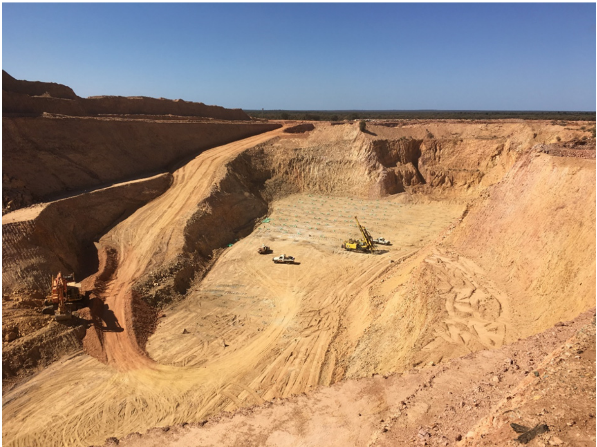
Figure 2. Mining at the Trouser Legs Gold Mine – Stage 1 Pit – Grade Control drilling in the base of the historic Anglo Saxon open pit – 350 metre RL (35 Metres Below Surface).
