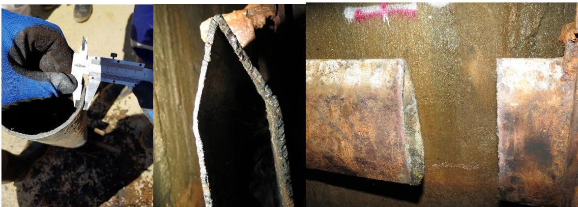
Figure 3: (LHS) Divider from submerged Bunton Set number 81 tested steel thickness to 5.0mm; (Middle) section through retrieved Bunton (RHS) location where bunton section was removed.
