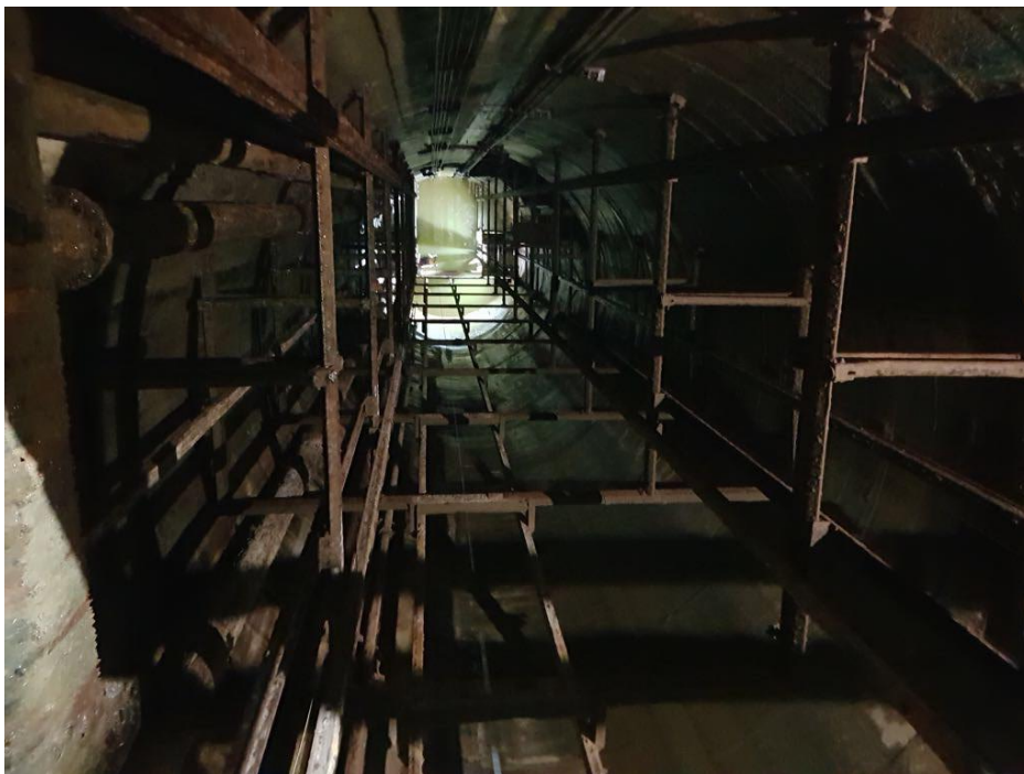
Figure 2: (Top) Plan-view schematic showing the configuration of the Hutchings Shaft and (Bottom) photograph of the Hutchings Shaft taken in January 2018 showing a similar plan-view perspective, with the accumulated water at the 350m Level.
