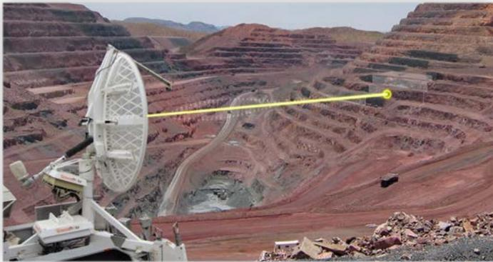
Radar-based monitoring solution
