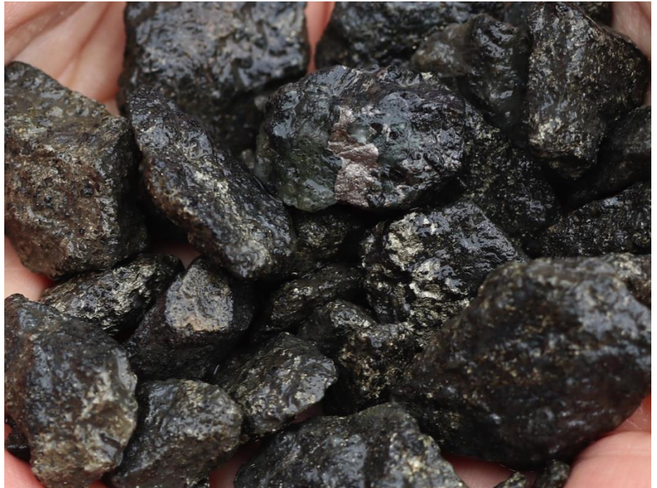
Pyrite & pyrrhotite sulphides from drilling north of Anomaly 3
