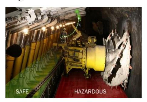
The integrated solution means that the location of tagged underground equipment and mining personnel is known accurately at all times. Real-time tracking of mining workers, roof support and excavation units improves worker safety and drives compliance. It also increases longwall operational efficiency, by safely accelerating work sequences and increasing operator flexibility.
