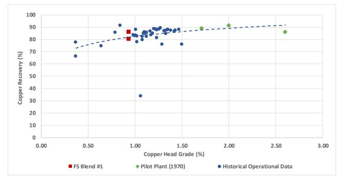
Figure 1: Graph showing the copper recoveries into marketable concentrates achieved for various head grades during historical mining operations ('Historical Operational Data')<sup>1,2</sup>, during 1970 Anglovaal pilot plant testing ('Pilot Plant (1970)') and during the latest locked-cycle testing ("FS Blend #1).
