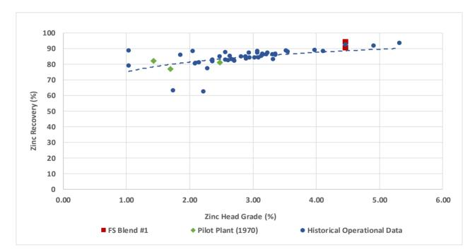
Figure 2: Graph showing the zinc recoveries into marketable concentrates achieved for various head grades during historical mining operations ('Historical Operational Data')<sup>1,3</sup>, during 1970 Anglovaal pilot plant testing ('Pilot Plant (1970)') and during the latest locked-cycle testing ("FS Blend #1).
