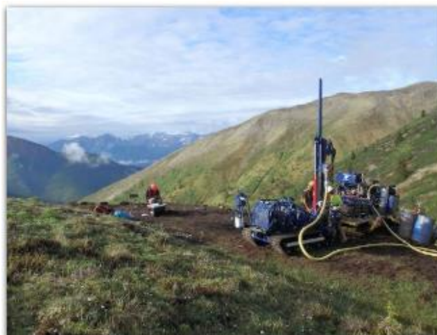
Figure 1: Scout – Rubber Track Mounted RC/RAB Drill
