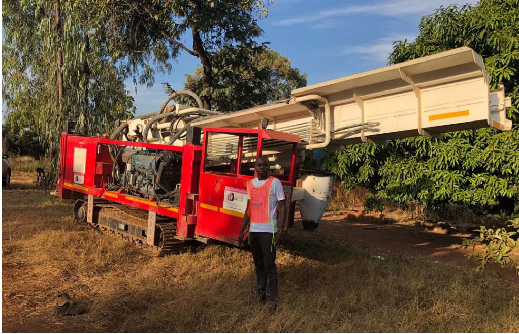
Figure 1: RC drill rig mobilized to site awaiting drill pad completion
