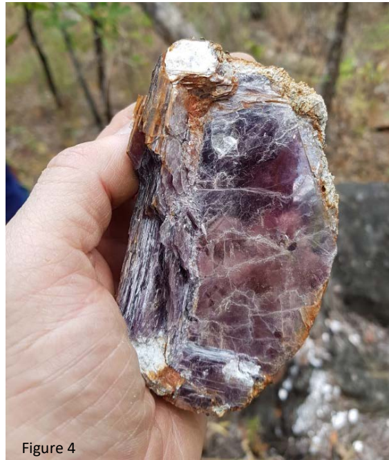
Figures 3&4: Figure 3 shows a close up of an outcropping high-grade lithium sample showing Li-bearing minerals such as spodumene, lepidolite and pink tourmaline from the Bonnyvale Prospect. Figure 4 shows coarse-grained Lithium mineralisation (Lepidolite) from the Hereford South Prospect.
