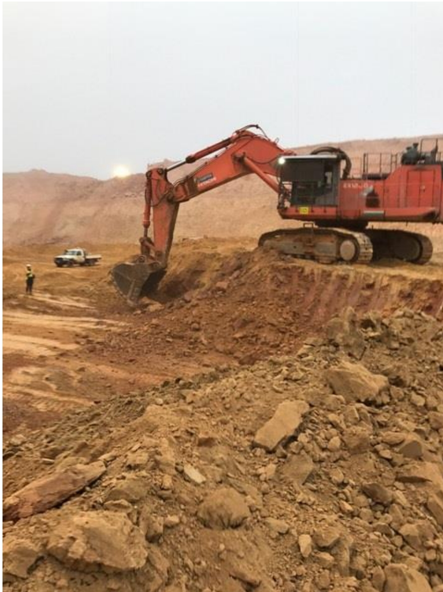
Figure 3. High Grade Ore Mining at the Trouser Legs Gold Mine – Stage 2 Pit – 350 metre RL (25 Metres Below Surface).
