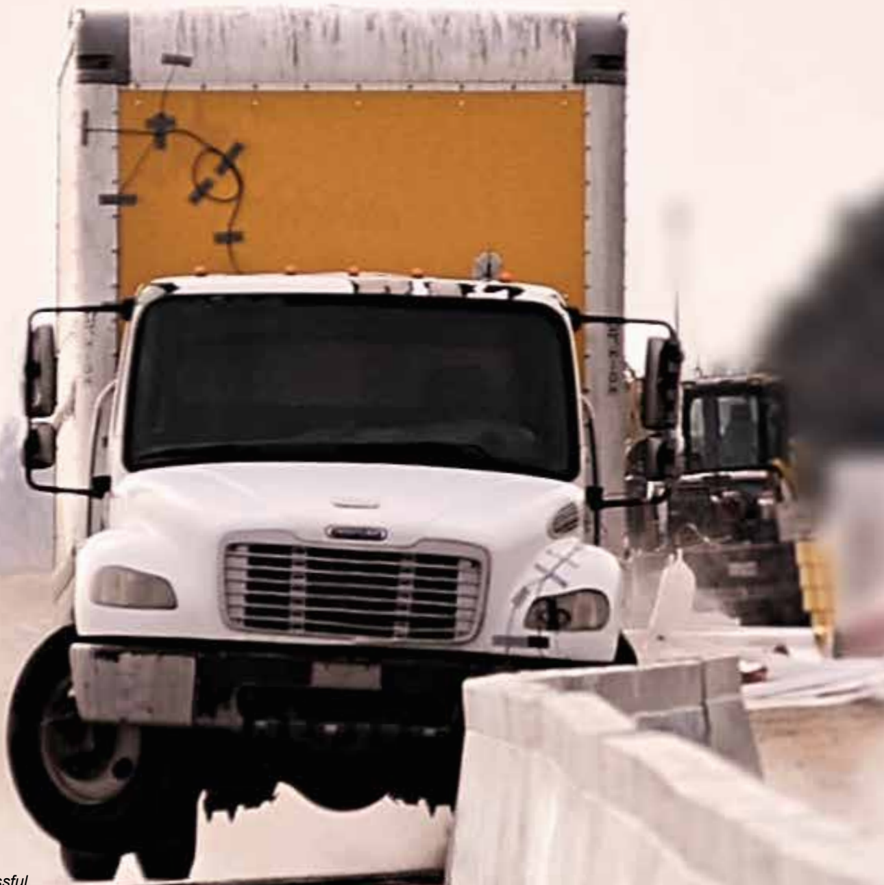
HV2™ Barrier successful TL-4 crash test - January 2018
