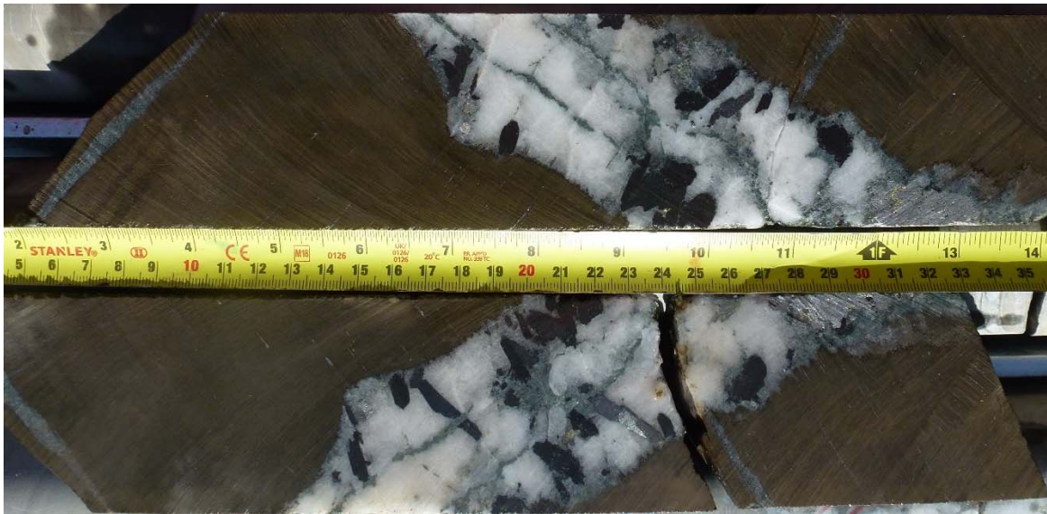
Figure 5 – CRD025: 412.5m – wolframite rich quartz vein
