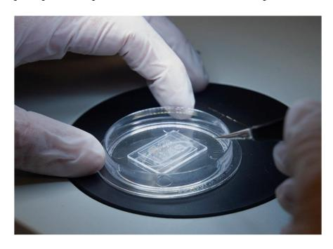
MEMS pressure sensors, ready for attachment to fibre optics and integrated into an implantable surgical device
