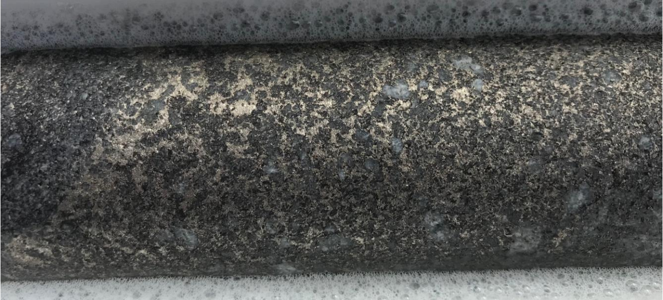
Photograph 2: Massive sulphide mineralisation from hole QDD0004, length 15cm, approximately 214 metres depth downhole
