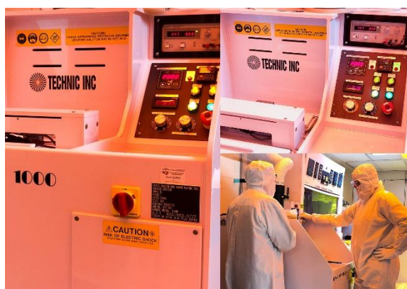
Automated Plating Tool – now creating features as small as 0.00225 mm
