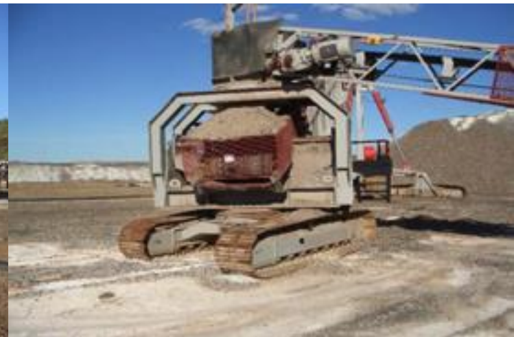
Figure 8 - Crawler-mounted radial stacker conveyor
