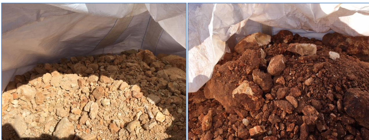
Figure 3. Bulk samples taken during the Quarter. The amount of iron present accounts for the colour difference.
