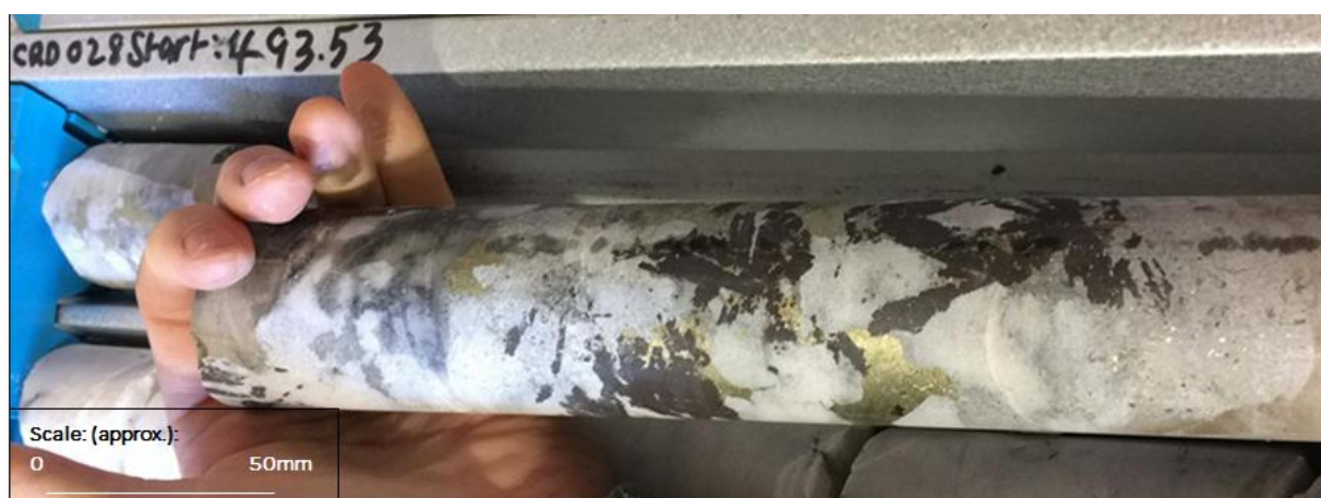
Plate 1: Well developed wolframite and chalcopyrite, in interval 493.16-493.91m, CRD028
