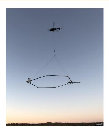
Figure 3: The SkyTEM<sup>™</sup> technology during survey operation (during the 2017 – 2018 regional survey).
