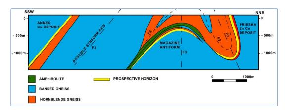
Figure 5: Simplified cross-section showing structural duplication of the Prospective Horizon – refer to the section line on Figure 4.
