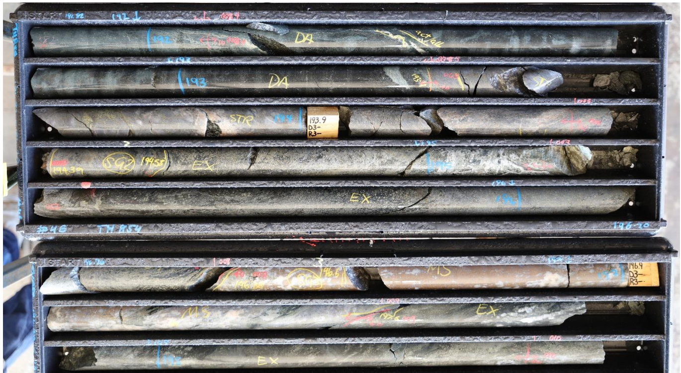
Figure 6 TH854 (4.20m @ 0.9% Cu, 6.1% Pb, 19.6% Zn, 0.3 g/t Au & 118 g/t Ag (31.1% Zn Eq.) from 193.40m to 197.60m down hole)
