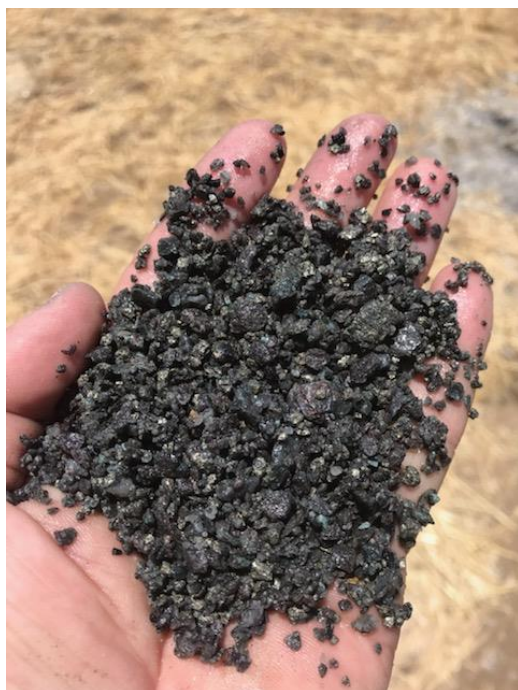
Figure 1: Sulphide mineralisation in ultramafic host rock. Drill hole QRC0168, 140-141m downhole.
