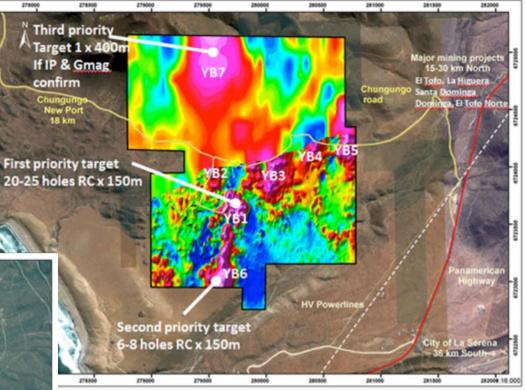
This image above shows the magnetic structures identified by the company's 3 ground magnetic surveys.
