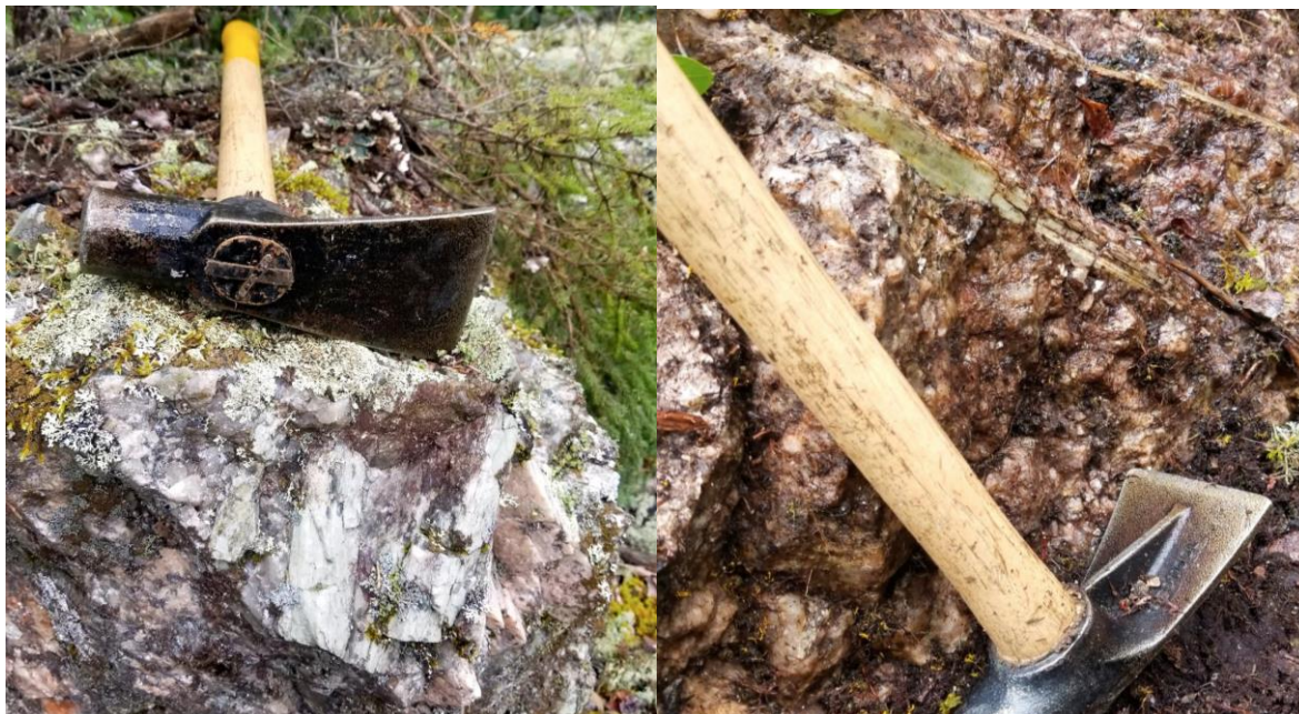
Photo 1.0 - SG1802 (104902)= 3.78 % Li 2 O – Grass River Pegmatite
