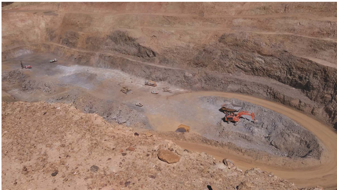
Figure 3. Trousier Legs Gold Mine – Looking West – 322.5 m Level – Stage 3 cutback.
