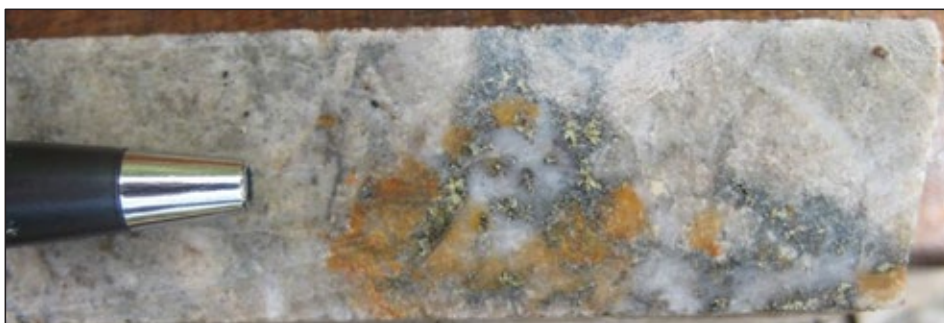
Figure 2-6: Silicified quartz-feldspar porphyry intrusion overprinted by quartz veins and quartz-chalcopyrite-pyrrhotite
