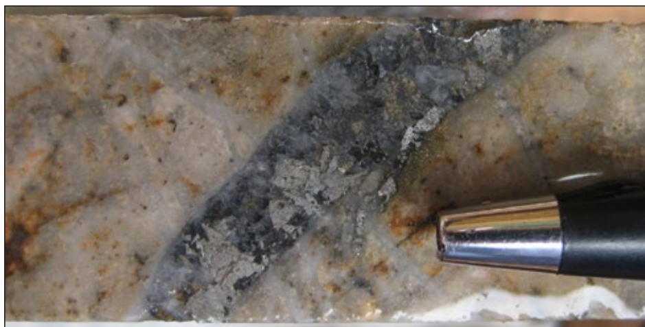
Figure 2-11: Quartz-arsenopyrite-pyrite vein overprinting earlier quartz veins in silicified feldspar porphyry intrusion
