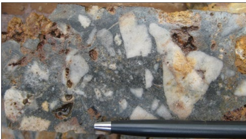
Figure 2-7: Angular to rounded fragments of intrusion and quartz vein in a breccia with a dark coloured matrix, previously described as quartz-tourmaline-rich
