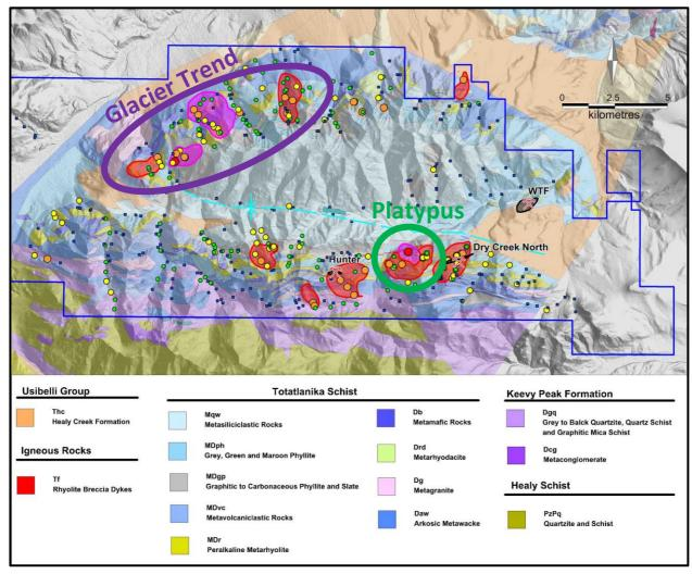
**Figure 3:** Location of high priority stream sediment geochemical anomalies including the Glacier Trend and Platypus target areas, on the DGGS geology map (after Freeman et al., 2016) and terrain surface with locations for the Dry Creek and WTF VMS deposits, and the recent Hunter VMS discovery.
