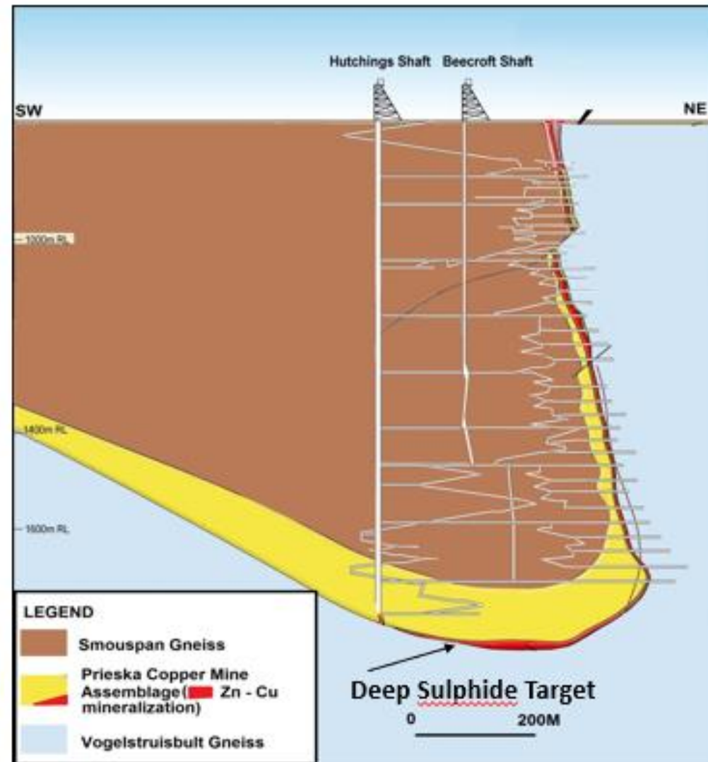
Figure 2A: Simplified geological section through Prieska Project showing structure and locality of the Deep Sulphide Target below the old workings.
