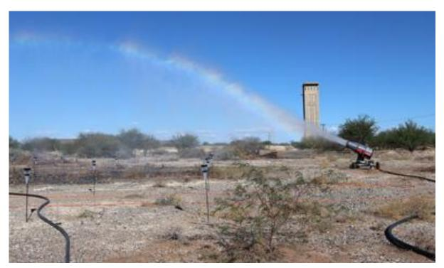
Figure 5: Feasibility study field trial of effectiveness of a 15kW evaporator at the Prieska Project. The planned pilot trials aim to test 75kW and 90kW units as the next phase of the program.
