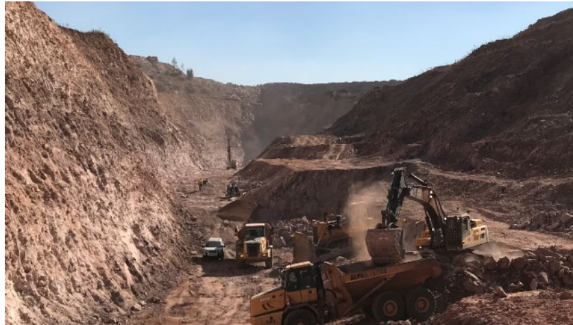
Image 3: An anomaly in the middle section of Pit 3 required to the remodelling the ramp to access the western end
