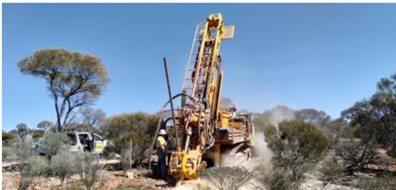
Figure 1: Photograph of aircore drill rig in operation during the recently completed drilling program test geochemical targets on the Monarch Gold Trend, Leonora East Project
