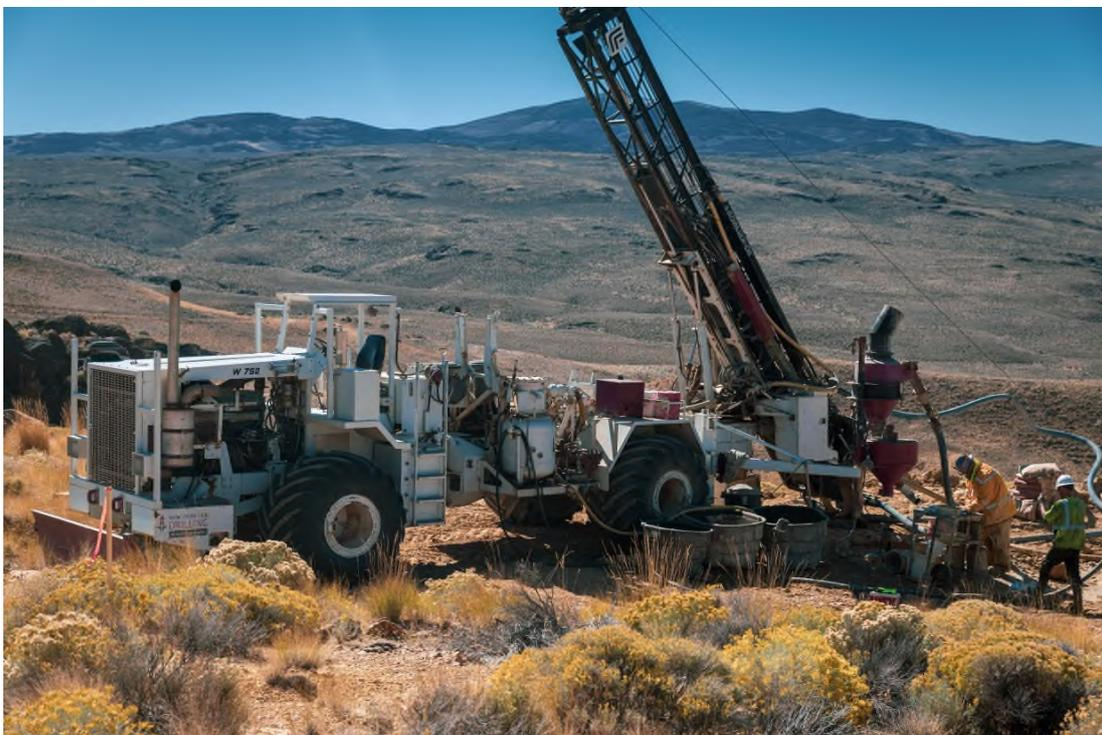
**Figure 1: RC drill rig on the first hole at the Bells Area – Hog Ranch Gold Property**
