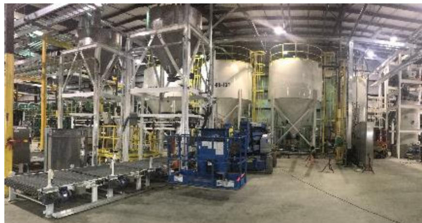
Intermediate storage bins, product bagging line, leach tank and filter press
