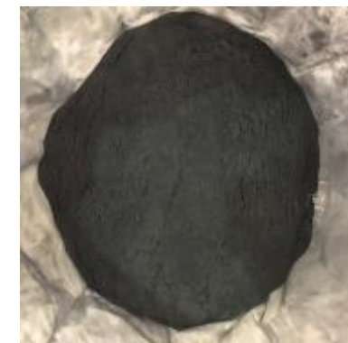
Milled unpurified spherical graphite for customer qualification
