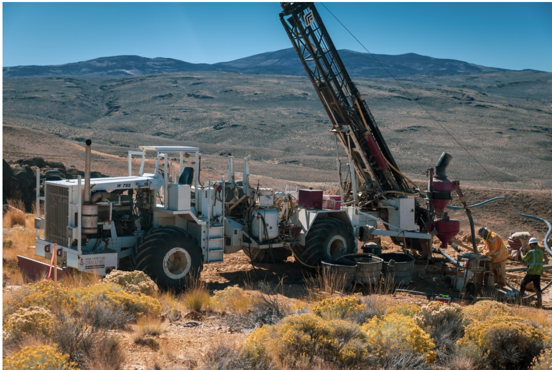
Figure 2: RC drill rig on the first hole at the Bells Area – Hog Ranch Gold Property
