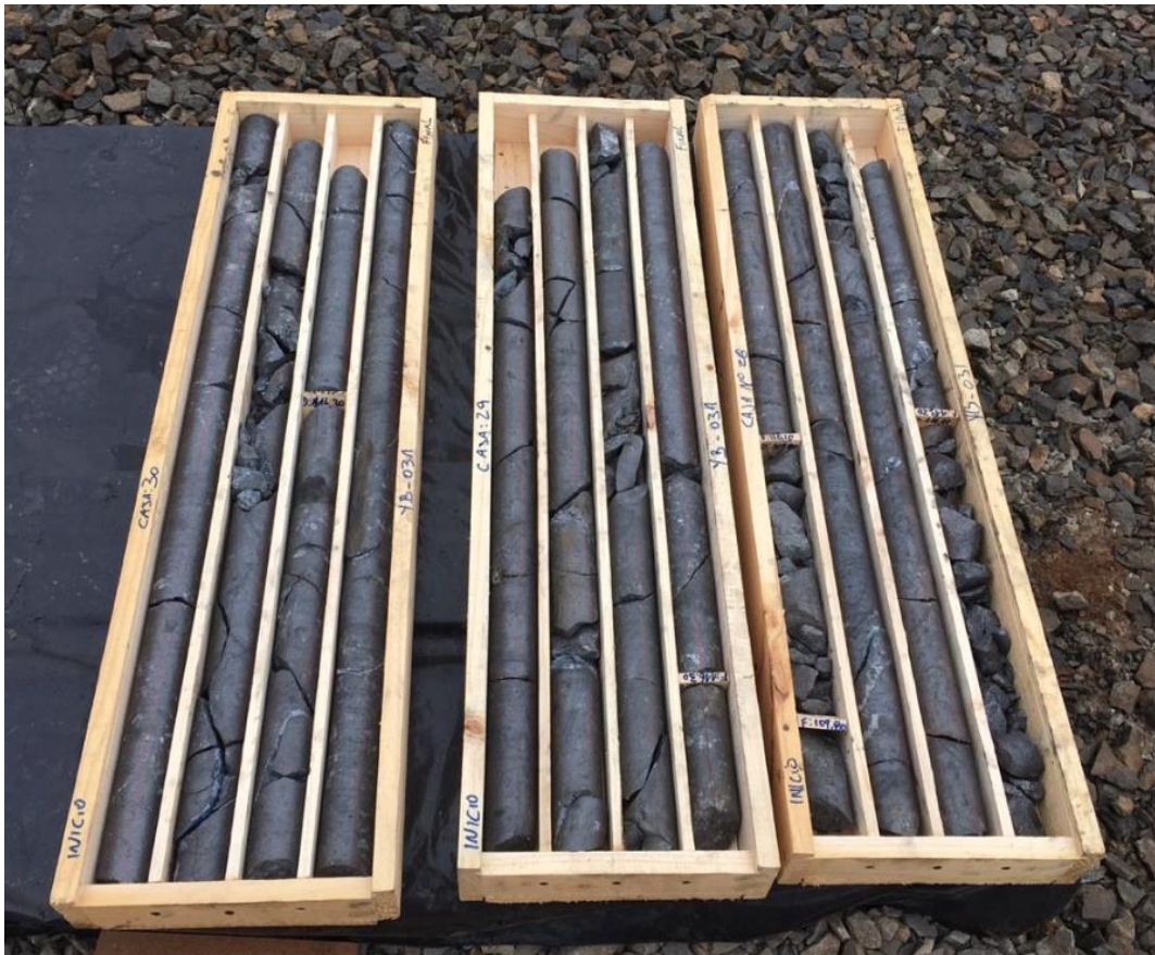
Figure 3 – Drill core trays showing black colouration, typical of high grade magnetite intersections
