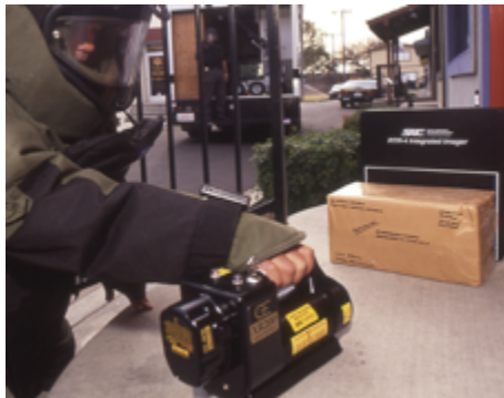
Above – Current bomb disposal X-ray imaging technique * EOD – Explosive Ordnance Disposal
