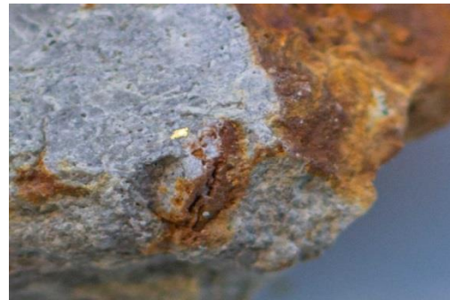
Photograph 2. Sample from the historic Fairleys open cut mine. Petrography offcut from Sample FC0025 1m @ 26.6 g/t Au (Sample approx.. 2.5 cm wide) – showing visible gold in silica sulphide altered sediment.
