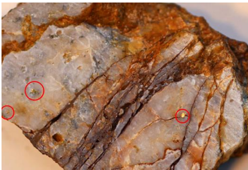
Photograph 1. Sample from the historic Miners Glory Mine. Petrography offcut from Sample 69972 0.2m @ 83.9 g/t Au (Sample approx.. 3cm wide) – red circles show visible gold occurrences.
