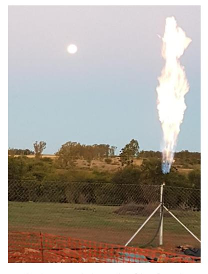
The gas was intersected under pressure in the morning of the 9 December 2019, after having drilled approximately 50 meters into the sandstone. The team on site has been flaring the gas
