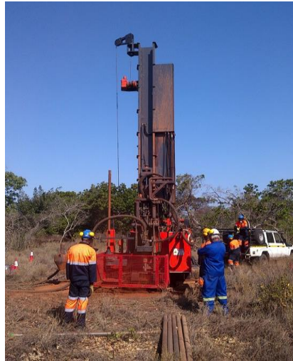
Figure 4: Aircore drill rig operation at Koko Massava.
