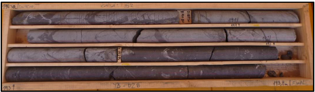
Figure 1 - Core tray 52 from diamond drill hole YB028 showing typical high grade magnetite mineralisation – interval 190.3m to 193.8m shown
