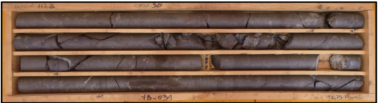
Figure 2 – Core tray 30 from diamond drill hole YB031 showing typical high grade magnetite mineralisation – interval 117.06m to 120.75m shown
