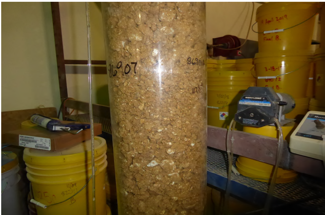
Figure 1: Column Leach Test at KCA Labs in Nevada, USA
