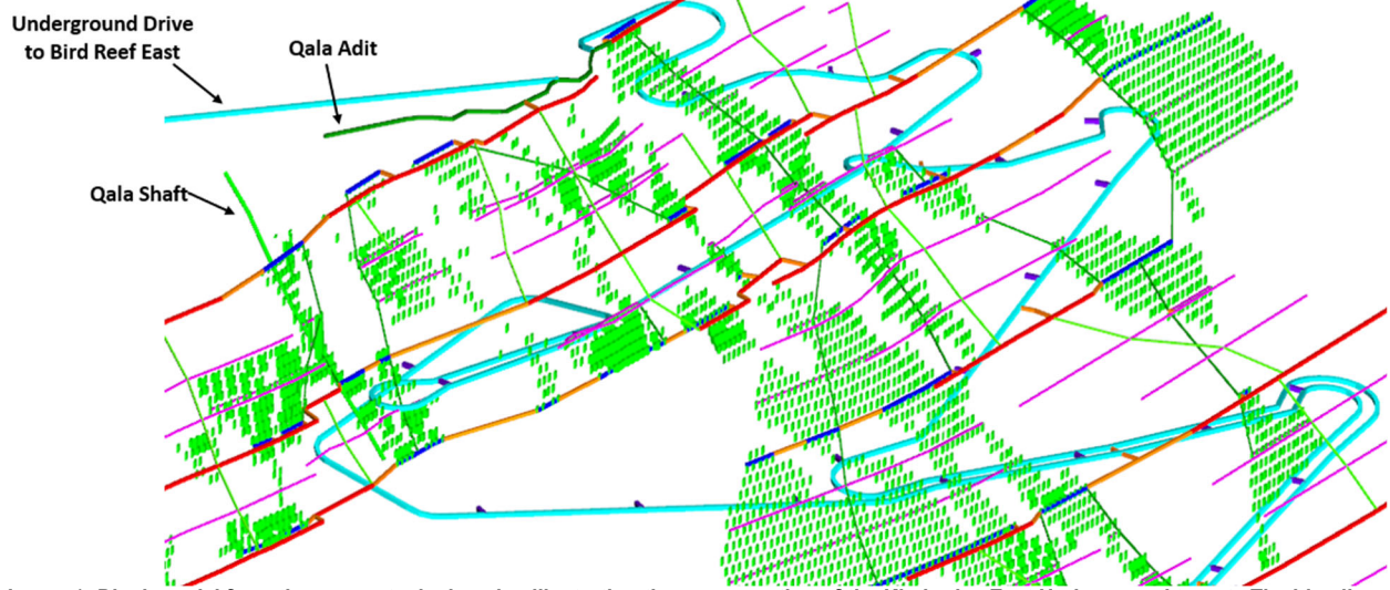
Image 1: Block model from the conceptual mine plan illustrating the upper section of the Kimberley East Underground target. The blue line dipping from the right side depicts development of the existing Qala Adit which runs at 10-15° which will enable trackless haulage.
