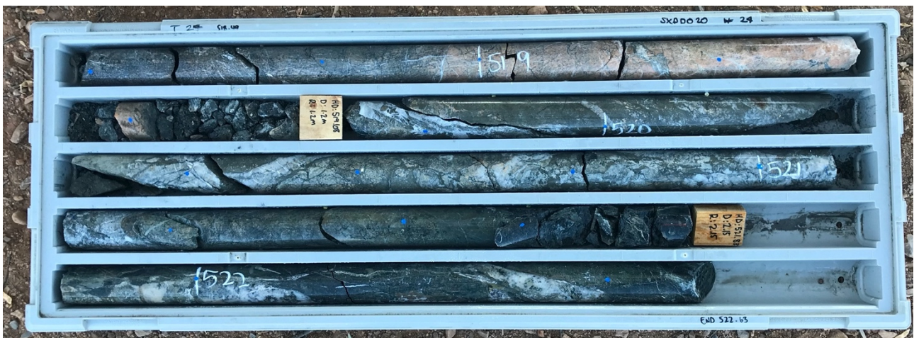
Figure 10: Drillhole SXDD020 (518.49-522.63m) drilled by SER late 2019; interval 520-521m assayed > 50g/t Au
