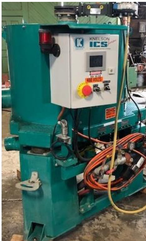
Figure 6 Knelson Concentrator and Screen acquired by Red River
