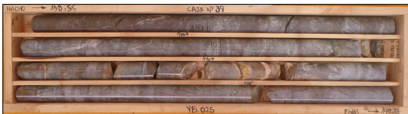
Figure 2 - Core tray 39 from diamond drill hole YB025 showing typical high grade magnetite mineralisation – interval 138.5m to 142.2m shown
