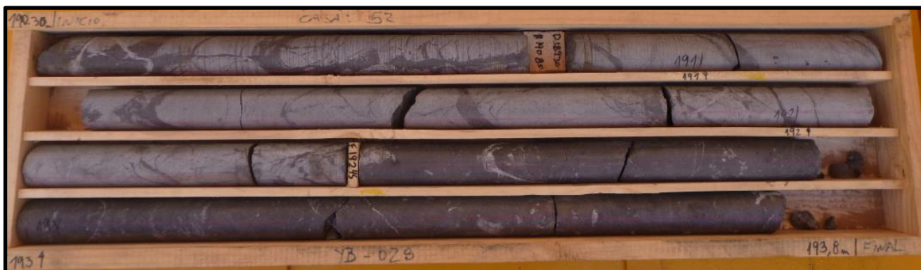
Figure 4 - Core tray 52 from diamond drill hole YB028 showing typical high grade magnetite mineralisation – interval 190.3m to 193.8m shown
