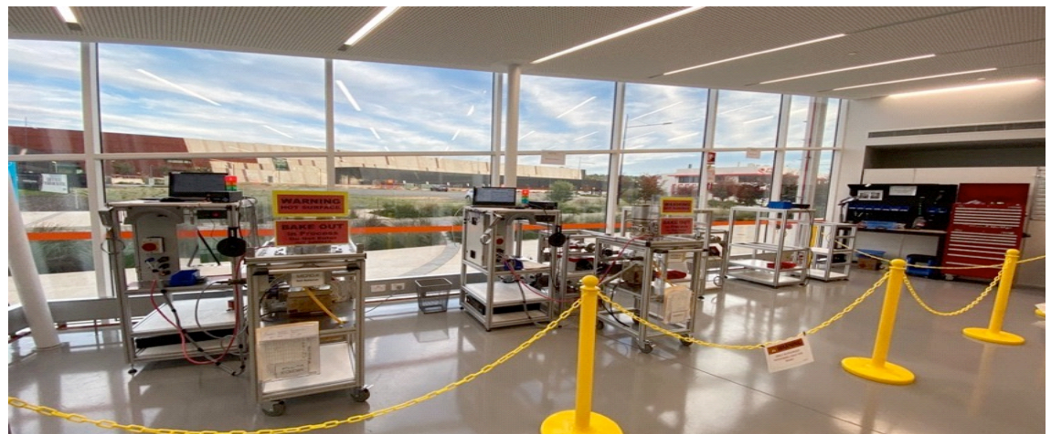
RIGHT: Doubling of automated X-Ray Tube bakeout cells from 2 to 4
