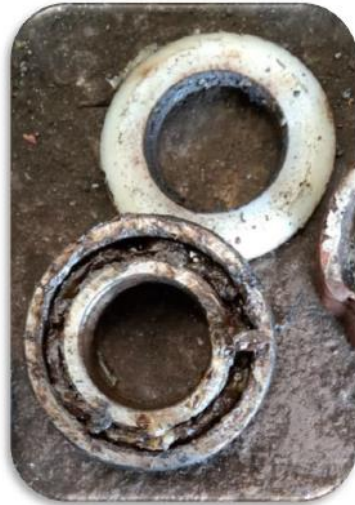
Removed bearing showing damage
