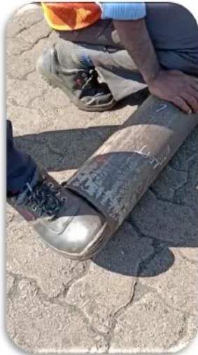
Roller removed and tested. Grinding noise noted while rotating the shaft
