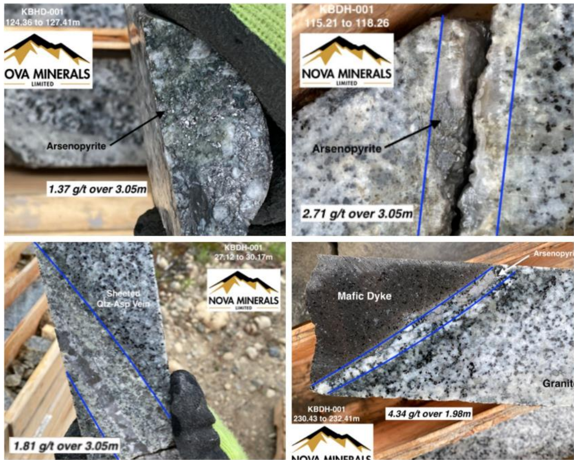
Figure 3. Core photos illustrating sheeted veins containing Arsenopyrite from higher-grade intercepts
