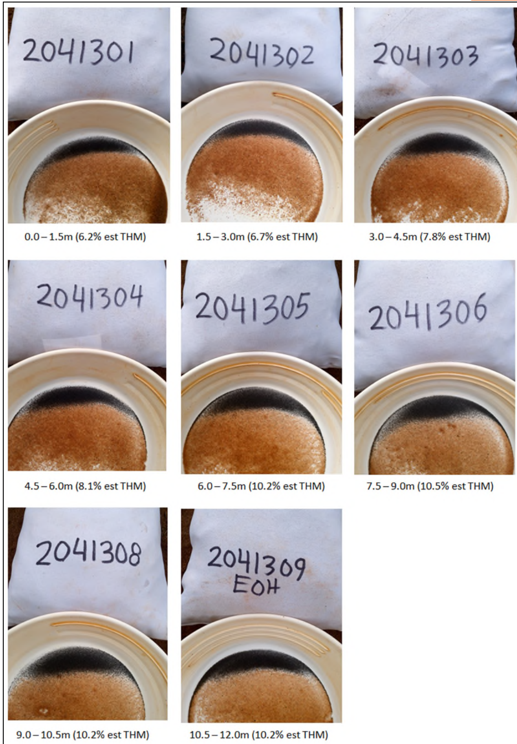
Figure 12: Field pan concentrate photos for auger hole 20CSHA413 showing the high grades intersected. Each sample shown is panned from the same volume of sand grab-sampled from the relevant 1.5m sample interval.
