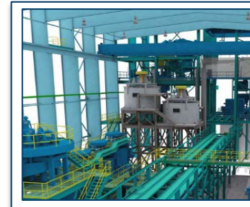
Engineering for cleaner and stack cells in progress
