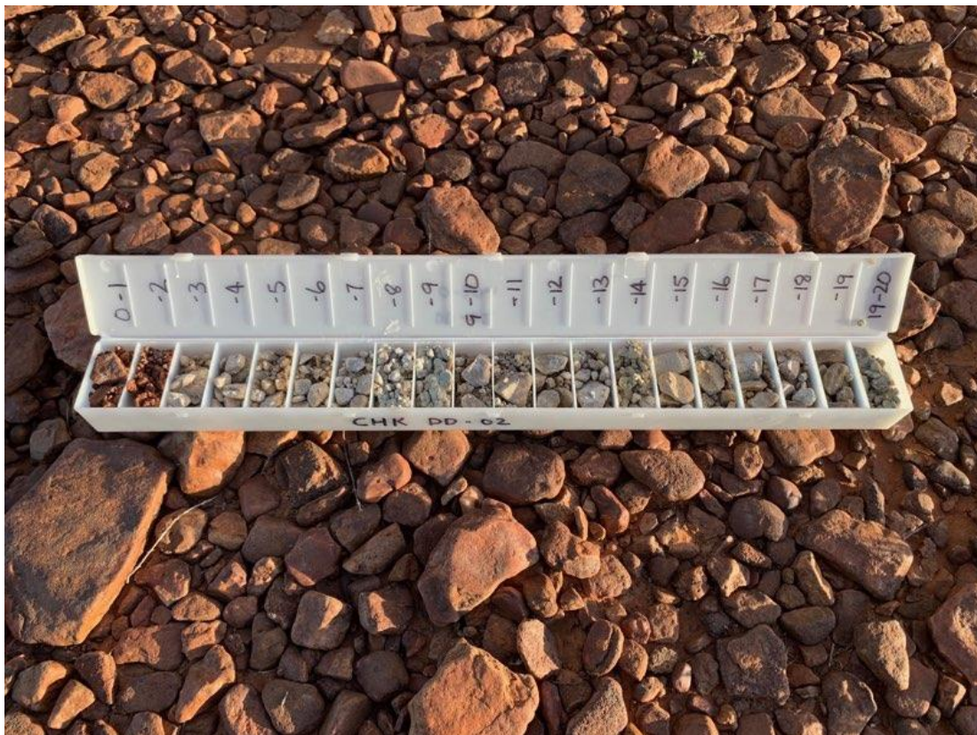
Figure 2: RC drilling chip samples from the top of drill hole HWDD_02
