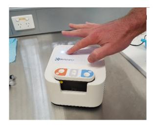
The Felix device incorporates a simple efficiently automated process that separates sperm in around 6 minutes. This is a marked improvement on the current sperm preparation techniques, density gradient centrifugation ("DGC") and "Swim up", currently used in IVF clinics. These techniques are consuming (each taking 30 to laborious. heavily minutes), and dependent on operator expertise.
